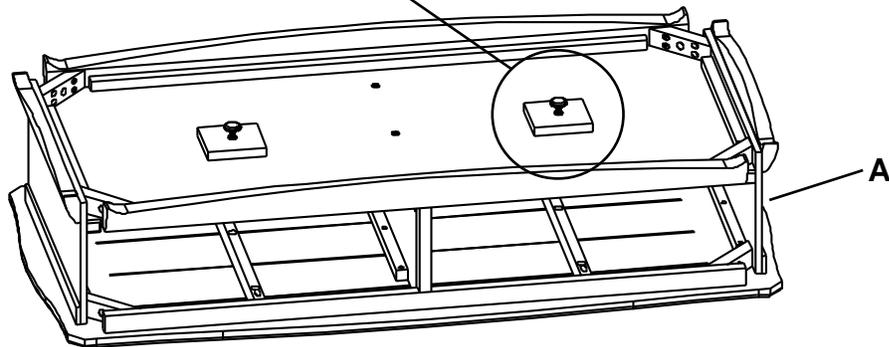
2. Place two Legs (B) at the front corners of the Case Assembly (A) making sure the drilled corners of the legs face toward the Corner Blocks. Insert two 3/8" x 2-1/2" Hex Bolts (R) with two Flat Washers (Q) through the Corner Blocks and into the leg and fasten securely. See Figures 2 and 2a. Repeat for the other two legs.
