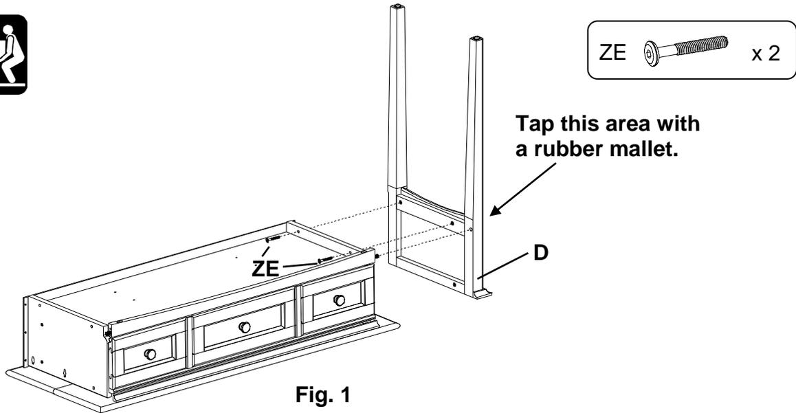
2. Using the Hex Wrench (ZH) attach the Right Side Assembly (E) to the case assembly with two 1/4" x 40mm Bolts (ZE). Fasten securely. Make sure the dowel is fully seated in place by tapping the Right Side Assembly (E) with a rubber mallet. See Figure 2.
