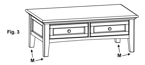
4. Place the table at its final destination. To level the table, rotate the Adjustable Glide (M) found at the bottom of each leg. See Figure 3.
