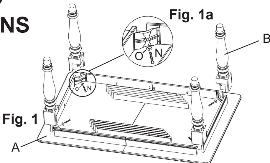
1. Place Top Assembly (A) upside-down on a clean, protected surface. Position Legs (B) on Top Assembly (A) outside of and against the corners of the aprons. Insert 3/8" x 2 1/2" Hex Bolt (N) through Washer (O) and Bracket, and screw into Leg (B). Tighten bolts. See Figure 1a. Turn your table upright. Retighten bolts (N) after first week of use.
