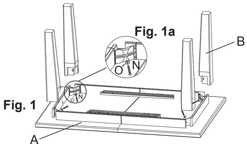
1. Place Top Assembly (A) upside-down on a clean, protected surface. Position Legs (B) on Top Assembly (A) outside of and against the corners of the aprons. Insert 3/8" x 2 1/2" Hex Bolt (N) through Washer (O) and Bracket, and screw into Leg (B). Tighten bolts. See Figure 1a. Turn your table upright. Retighten bolts (N) after first week of use.
