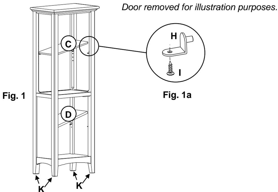
2. Place the tower at its final destination. Rotate the Adjustable Glides (K) found at the corners of the unit until the unit is level. See Figure 1.
