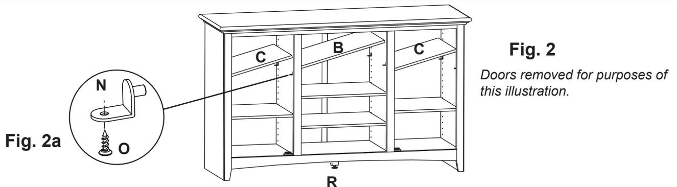
2. To move the Adjustable Shelves (B & C), remove the #6 x 1/2" Undercut Screws (O) and the Shelves (B & C). Reposition the Shelf Brackets (N) to the desired positions, replace the shelf and insert the screws. See Figures 2 and 2a.
