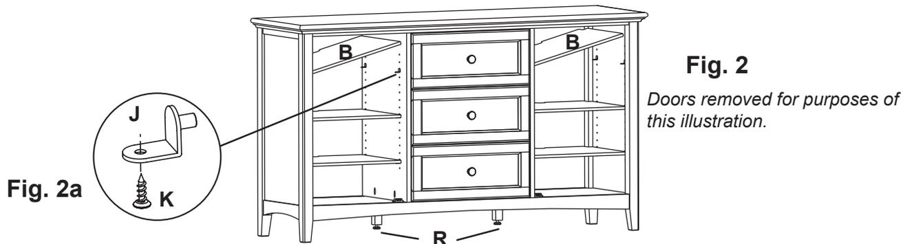
2. To move the Adjustable Shelves (B), remove the #6 x 1/2" Undercut Screws (K) and the Shelf (B). Reposition the Shelf Brackets (J) to the desired positions, replace the shelf and reinsert the screws. See Figures 2 and 2a.
