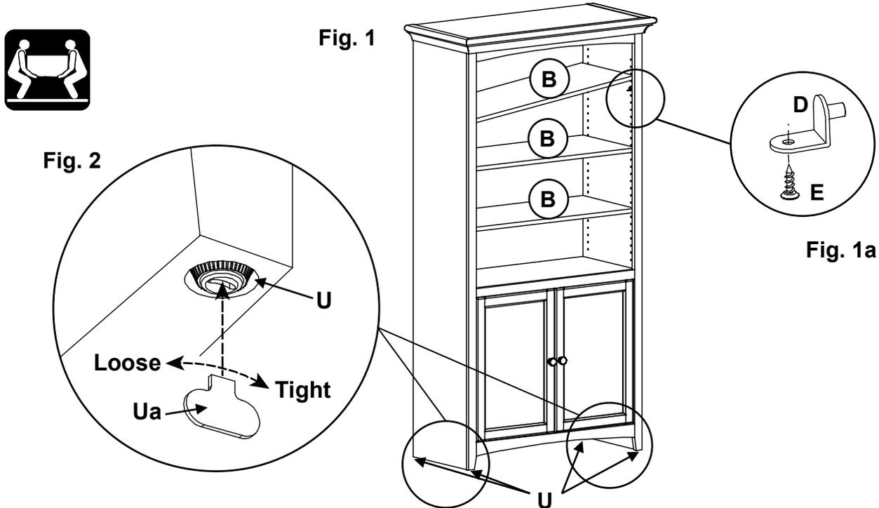
**2. Place the unit at its final destination. Use the Level Adjustment Key (Ua), found in the Zip bag taped to the Owner's Manual and Safety Guide to rotate the Slotted Levelers (U) on the bottoms of the legs until the unit is level. See Figures 1 and 2.**
