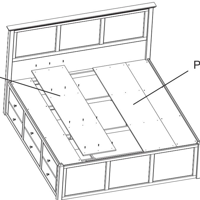
8. Place Deckboards (P) as shown in Fig. 7 and secure with #8 x 1" Screw (E).
