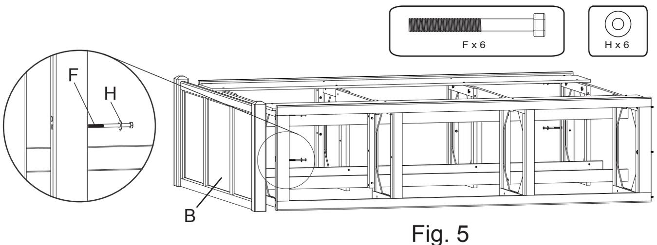
5. Assemble the Footboard (B) to the Pedestal Assembly as shown in Fig. 5. using 1/4" x 3" Hex Bolt (F) and Washer (H).
