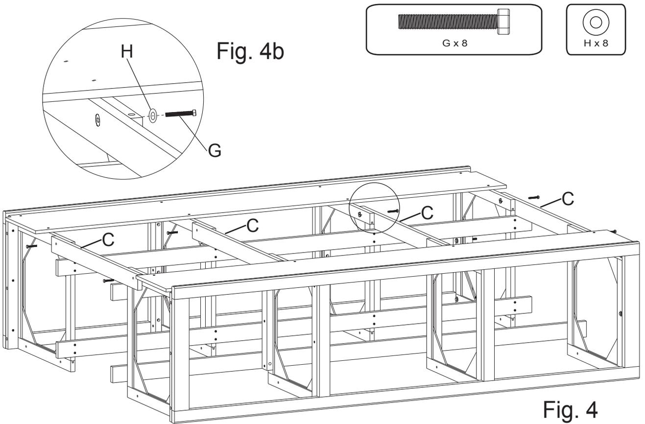
4. Place 4 Trestles (C) in between Pedestals and insert 1-1/4" Hex Bolt (G) and washer (H) as shown in Fig. 4b. Finger tighten only.
