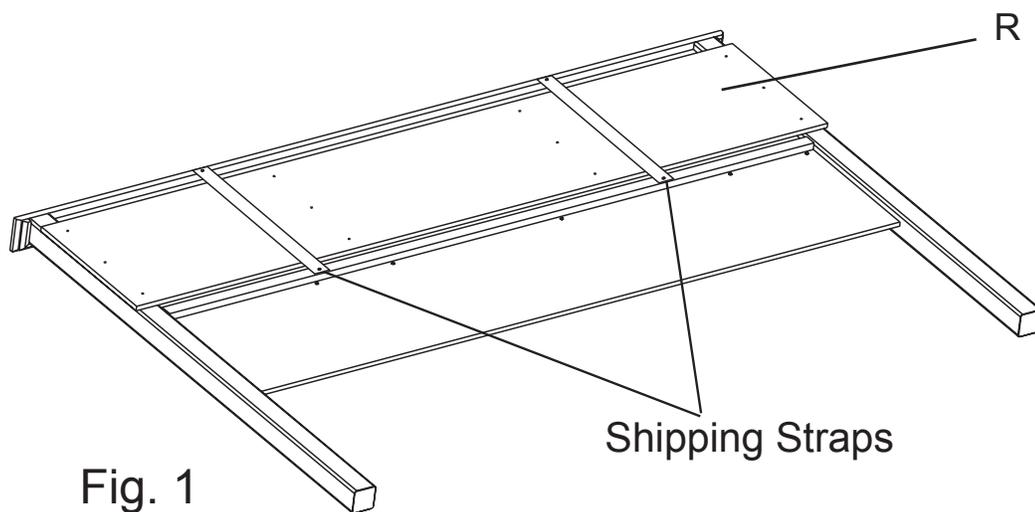
1. Remove the Trestles and Center Deckboard (R) from the back of the Headboard as seen in Fig. 1 and place them off to the side.
