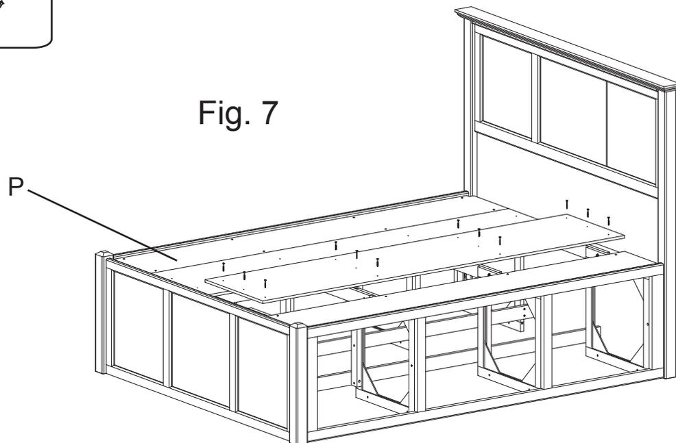
8. Place Deck Boards (P) as shown in Fig. 7 and secure with #8 x 1" Screw (E).
