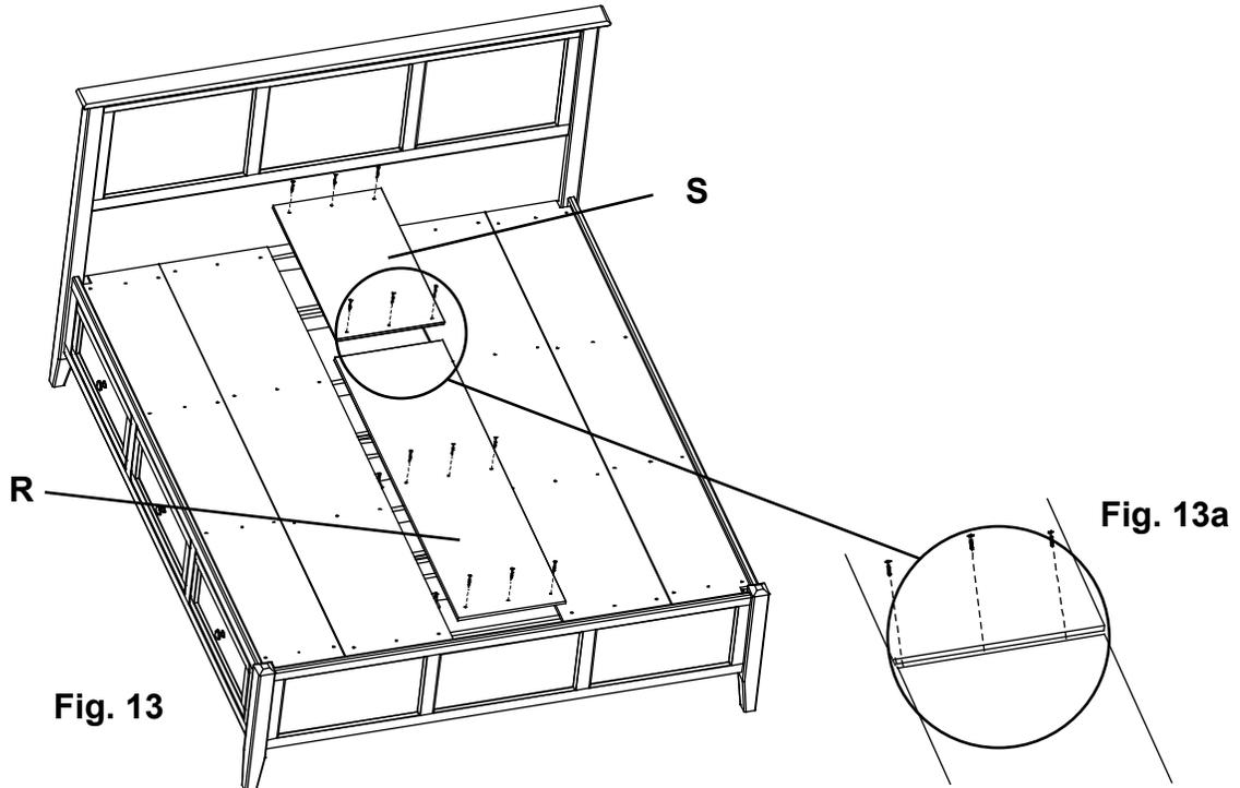
Place three #8x1-1/4" Black Screws (E) along the seam between the Deckboards (R) and (S). See Figure 13a.
