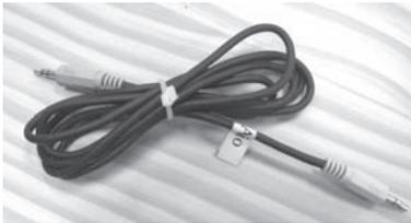
mini-pin/mini-pin cable **Fig. A**
