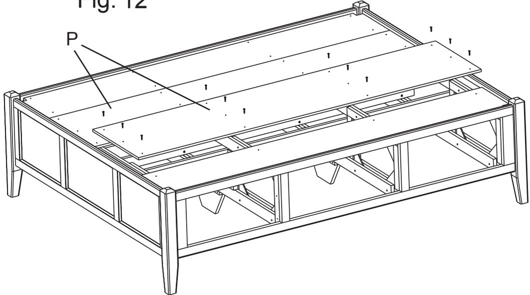
12. Place Deckboards (P) as shown in Fig. 12. There should be a small gap between each deckboard. Secure with #8x1¼" Screw (E).
