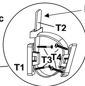
Pull the Nylon Restraint Strap (T2) tight so there is no slack.
